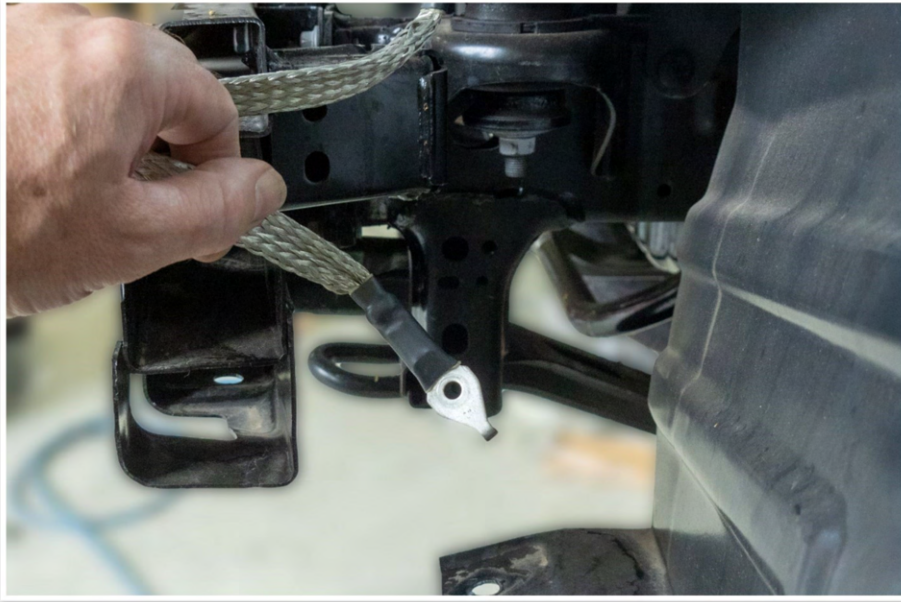
19. Remove the earth strap from the left hand side chassis rail.
