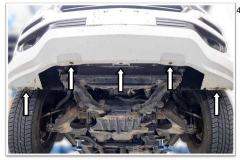
The bottom of the bumper bar is held in place with five fasteners, remove these and discard as they are no longer needed.
