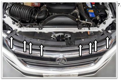
Remove the Torx screws that secure the top of the grille. Keep these as they are needed when refitting the grille.
