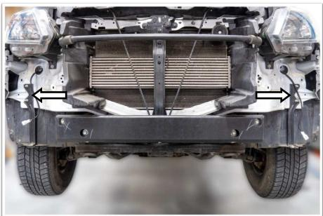
Remove the bumper bar retaining brackets from the vehicle. These can be discarded as they are no longer used.
