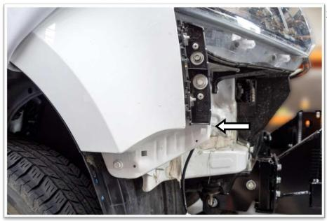
20. Trim the outer bumper bar retaining brackets in line with the bottom of the guards.
