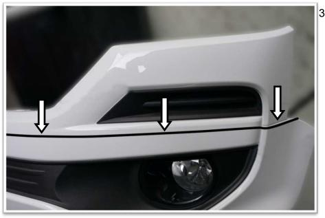
38. The bumper gets trimmed in a straight line from the crease where the outer bumper changes from vertical.
