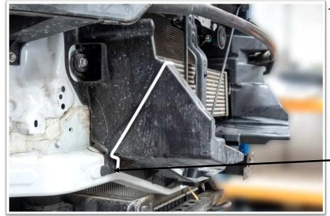
19. The radiator air guides need to be trimmed to allow for the winch mount. Trim them as shown opposite. Make sure to keep the bottom fastener.
