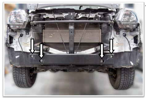
18. Remove the intrusion beam.
