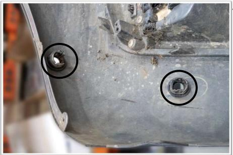
45. Remove the parking sensors and parking sensor brackets from the bumper bar. Again noting the location and orientation of the brackets as they are different and will only fit into the bull bar in their original location.
