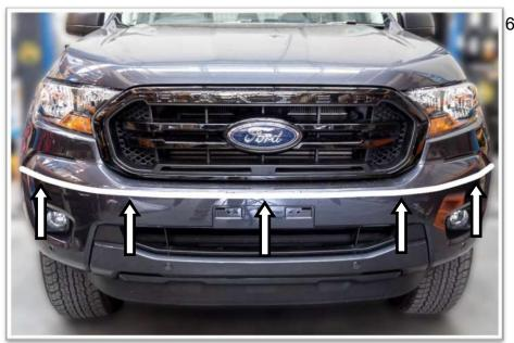
The cut line across the front will depend on what model vehicle you have. Some will cut the bumper, others will cut through the grille, mark 10mm down form the crease in the bumper bar.
