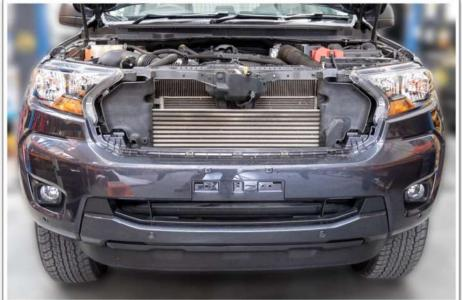
11. Release the clips along the lower part of the grille and remove.
