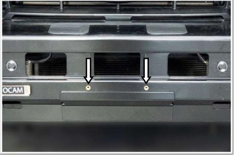
78. If there is no winch fitted, fit the number plate directly to the bar.
