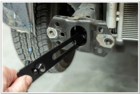
35. Insert the nut plate (item # 5) into the chassis.
