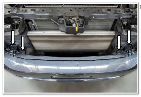
Remove the four (two each side) plastic clips that secure the bumper. Keep these for reinstalling the trimmed bumper bar.
