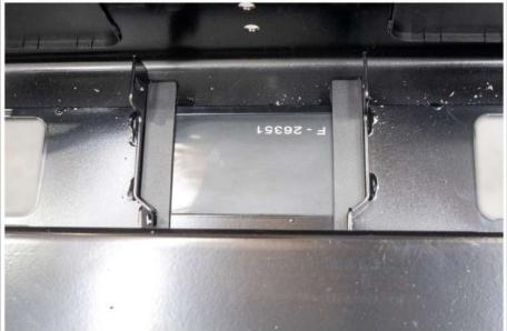
50. Fit the radar cover plate (item # 10) to the bull bar. The textured surface to the front of the bar.
