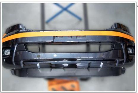
46. Using a air saw or multi tool, trim the bumper as previously marked.
