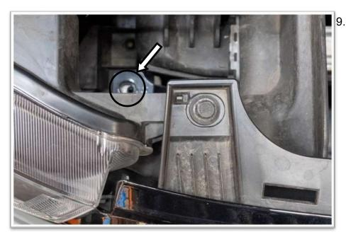
There are two hex bolts (8mm head) located behind the inside of the headlights. You will need a long extension to get to them. Remove these two bolts (one either side). Keep for reinstalling the bumper bar.
