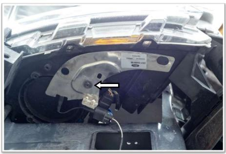
Refit the DAB antenna to the underside of the headlight.
