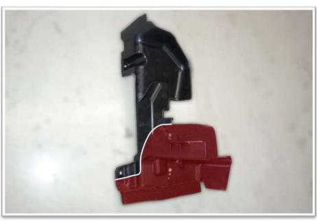
33. Trim the bottom section of the radiator air guides as shown.
