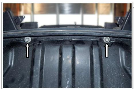
28. Remove the bolts that attach the OE stone tray to the intrusion beam. Loosen the rear bolts and remove the stone tray.
