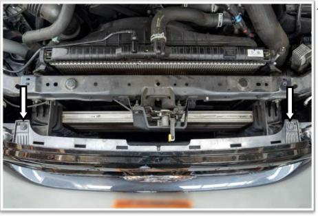
10. Remove the two M6 hex bolts securing the top of the grille.
