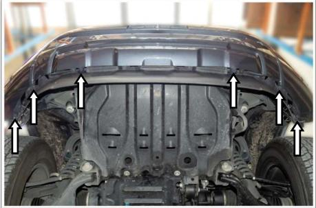
15. From underneath, remove the fasteners that hold the bumper bar in place.
