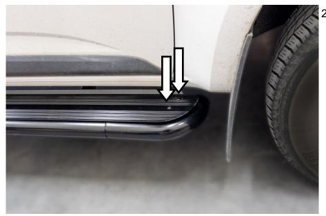
Remove the front two fasteners securing the tread plate to the step return. Keep the fasteners.
