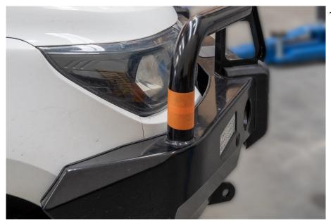
With the vehicle in a suitable location, start by applying masking tap to the outer loops of the bull bar. This is to protect the finish.
