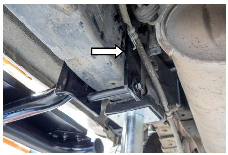
8. For the rear right hand side, use the RH spacer plate (item # 8), M10 x 130mm hex bolts, crush tubes (item # 10), M10 spring washers, flat washers and M10 hex nuts to secure to the rear mount of the side step.
