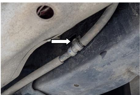
11. At the rear left hand side, remove the handbrake cable fastener.
