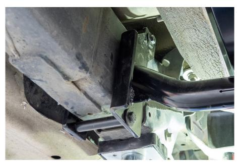
14. Secure to the rear bracket using M10 x 130mm hex bolts, crush tubes (item # 10), M10 spring washers, flat washers and M10 hex nuts.
