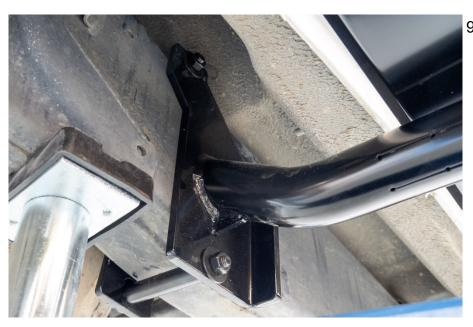
With the side step fitted to the vehicle, tighten the front mount first, then with the step parallel to the sill of the vehicle, tighten the rear mount.
