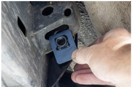
Insert one of the M12 nut plates (item # 9) into the lower hole in the chassis bracket.
