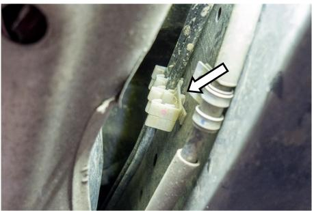
12. Unclip the hard line bracket form the chassis rail.
