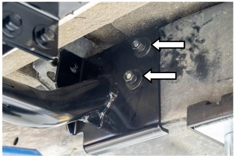
4. Lift the side step into place, secure front of the step using the previously installed U-bolt, M10 spring washers, flat washers and hex nuts. Leave loose.
