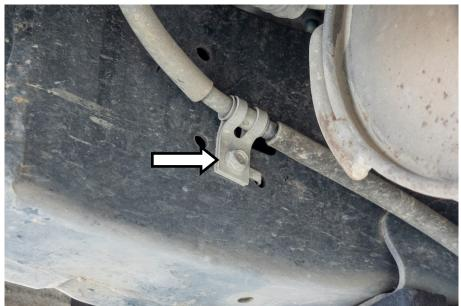
7. Remove the bolt from the handbrake cable at the rear.
