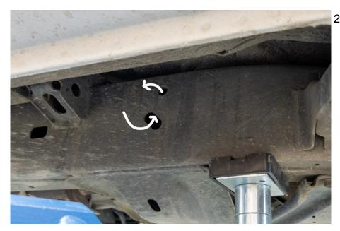
2. At the front of the vehicle insert a U-bolt (item # 12) into the lower slot and out through the hole above.
