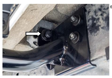
Secure the front mount to the chassis bracket using a M12 x 30mm hex bolt, M12 spring and flat washer. Do not tighten yet.
