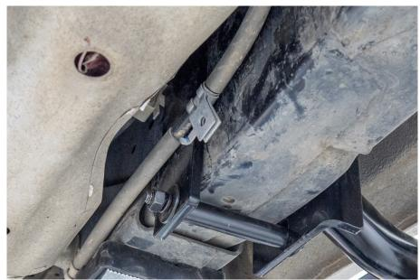
13. Position the left hand spacer plate (item # 7) between the hard lines and the chassis.
