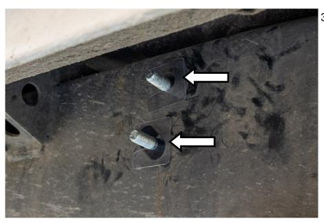
3. Use the plastic clips (item # 11) to hold the U-bolt in place.
