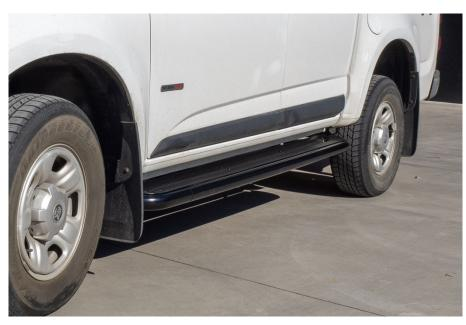
15. With the left hand side step fitted to the vehicle, tighten the front mount first, then with the step parallel to the sill of the vehicle, tighten the rear mount.
