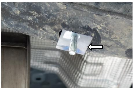
26. Secure the T-bolt in place with a plastic retainer.
