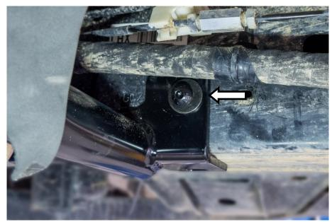
13. Secure the left hand side front mount to the side of the chassis rail using the M10 button head bolt, M10 spring and flat washer.
