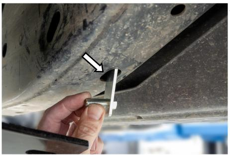
8. Insert one of the T-bolts (item 4) into the hole at the rear of the chassis rail, plate first, and manoeuvre so the bolt is protruding from the hole.
