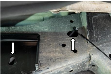
17. Insert another M10 bolt on a wire into the oval hole to the rear of the mount.
