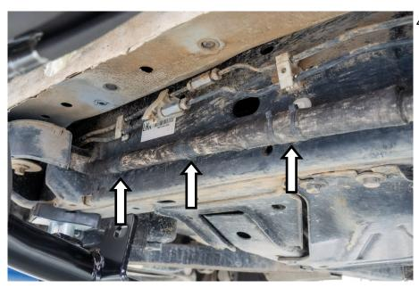
On the left hand side, carefully pry the loom away from the chassis.
