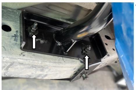
18. Secure the two M10 bolts on wire with M10 hex nuts, M10 spring and flat washers.
