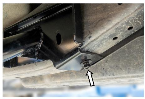
Lift the rear of the side step to meet the previously inserted Tbolt. Secure using a M10 hex nut, M10 spring and flat washer.
