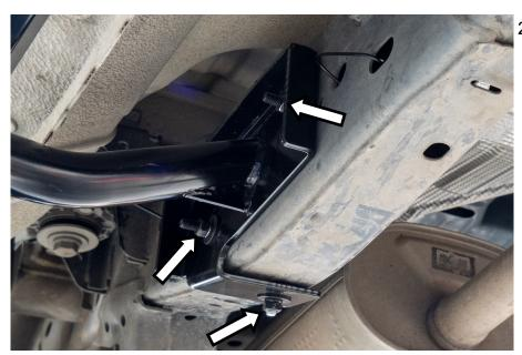
27. Insert the remaining two bolts on wire into the chassis. Secure the three bolts with M10 hex nuts, M10 spring and flat washers.
