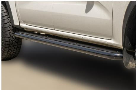
32. Align the step so that it is parallel to the sill and tighten the fasteners to the correct torque.
